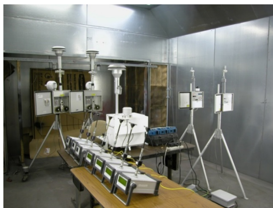
Figure 5.4.5. Various air quality monitors have been tested by the National Technology and Development Program for their suitability to wildland fire application.
