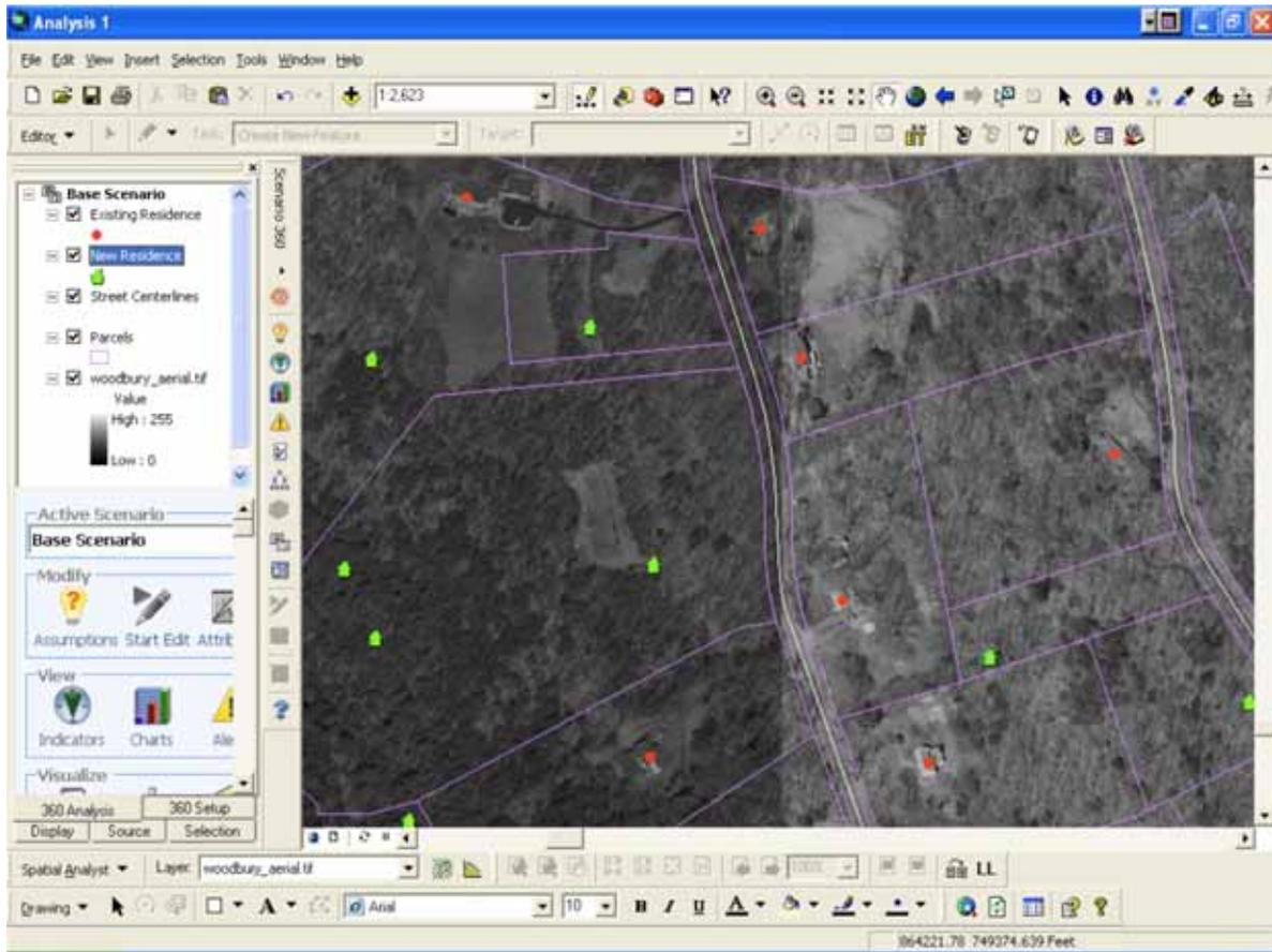
Figure 3. Screen capture of a the *CommunityViz* buildout program. In the window shown above the purple lines show parcel boundaries, red dots show existing buildings, and green houses potential future building locations. The aerial photo underneath the data layers shows the existing use of the land.
