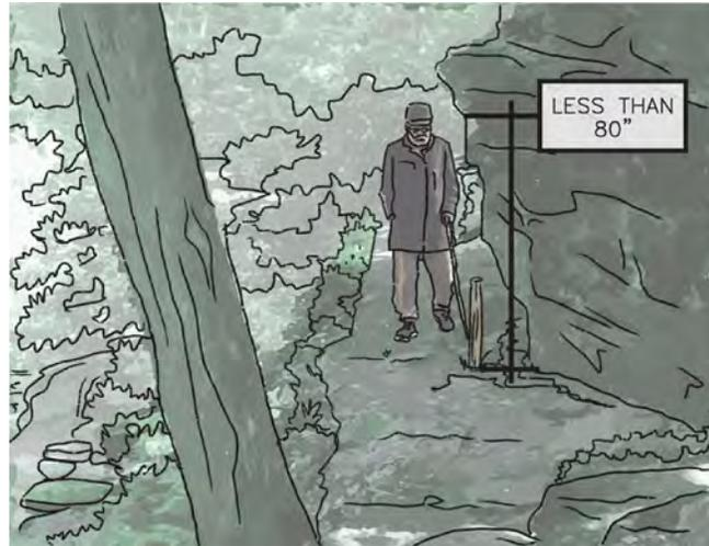
If vertical clearance is not possible (for instance as with a naturally occurring, overhanging rock formation protruding into the trail treadway, as shown in the illustration), a cane-detectible barrier to warn visually impaired trail users could be warranted.
