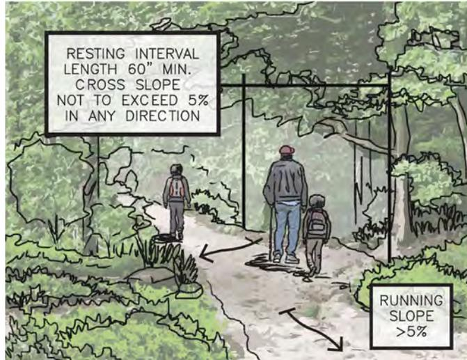
Resting intervals are required at the top and bottom of each trail segment that exceeds 5% in grade. The Outdoor Guidelines permit Resting Intervals and Passing Spaces to overlap.
